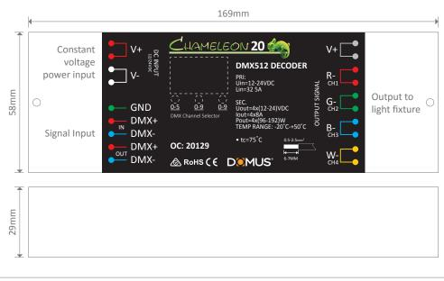
Note: -The lamp must be installed by professional electrician -Ensure the power supply is switched off before fitting this product
